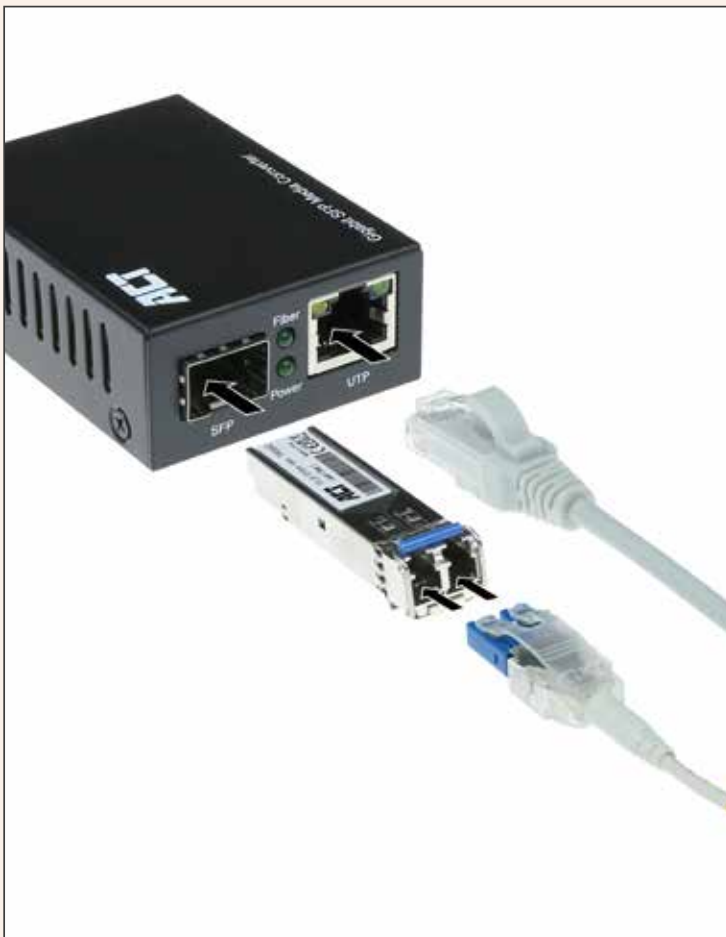
On the right, a network cable connected directly to the media converter. On the left, a fiber optic patch cable connected to the SFP module, the SFP module is plugged into the media converter.
